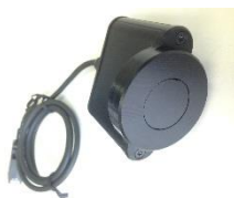
Non-destructive probe Meas.Spot : \phi 25 mm
