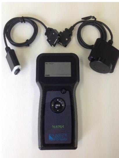
Mainbody + Contact probe(Left) + Non-destructive probe(Right)
