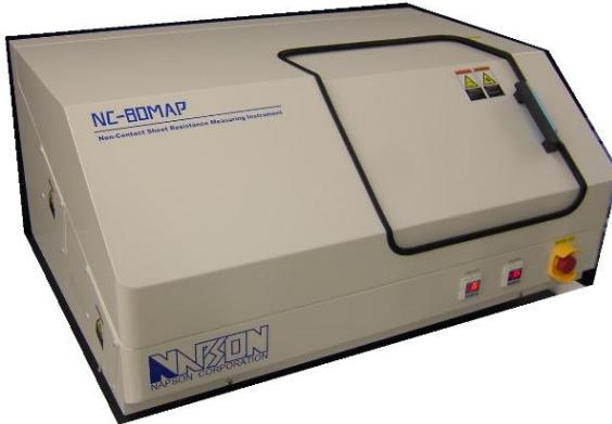
The NC-80MAP measures sheet resistance for GaAs ,GaN, SiC wafer and metal layer etc. without contacting (Eddy current measurement method). It provides high accuracy/high tact measurement.
